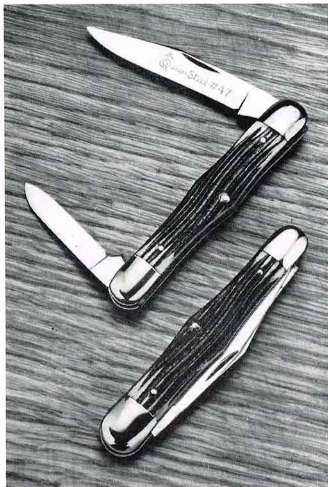
No. 47 Balloon Pattern — Two Blade Pen Knife. Genuine Frontier Bone stag handle. Made of Queen Steel. Will not rust or stain and because of our secret tempering process, it will stay sharp far longer than other knives. Nickel Silver double bolsters, brass linings. Clip blade 2\frac{7}{16} inches long with 2\frac{1}{8} -inch cutting edge and pen blade 2\frac{3}{8} inches long with 1\frac{3}{8} -inch cutting edge. 3\frac{1}{2} inches overall.
