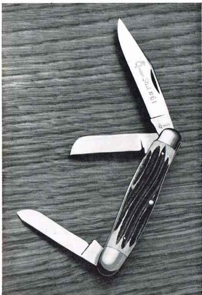
No. 61 — Stockman's Pattern — Three Blade Serpentine medium size stockman's knife. Genuine Frontier bone stag handle. Made of Queen Steel. Will not rust or stain and because of our secret tempering process, it will stay sharp far longer than other knives. Nickel silver double bolsters, brass linings. Clip blade 2\frac{3}{4} inches long with 2\frac{3}{8} -inch cutting edge, sheep's foot blade 1\frac{13}{16} inches long with 1\frac{5}{8} -inch cutting edge, Spey blade 1\frac{5}{8} inches long, 3\frac{5}{8} inches overall when closed.
