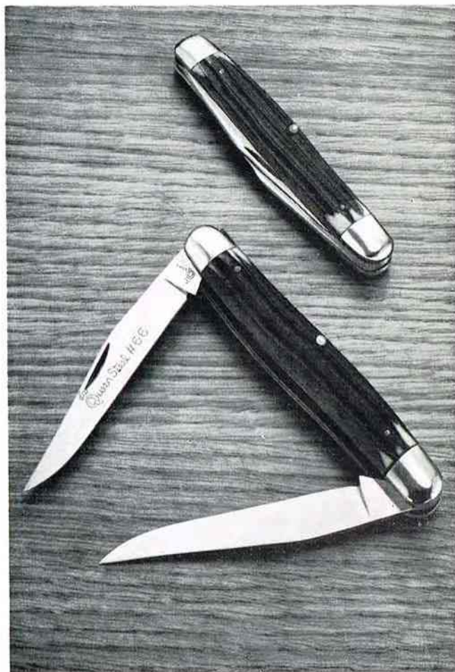
No. 66 Muskrat Pattern —Two blade pocket knife. Genuine bone stag handle. Made of Queen Steel. Will not rust or stain and because of our secret tempering process it will stay sharp far longer than other knives. Nickel Silver double bolsters, brass linings. Two clip blades, each 3-inches long with a 2 \frac{3}{4} -inch cutting edge. 4-inches long when closed.
