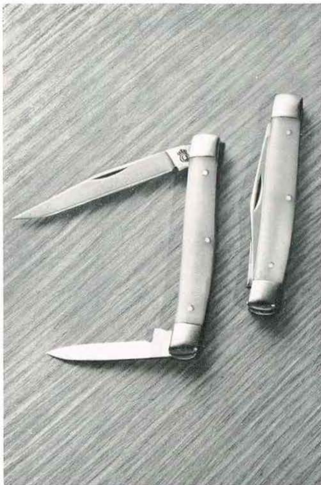
No. 42 Small Two Blade Serpentine Pattern — Amber handle. Made of Queen Steel. Will not rust or stain and because of Queen's secret tempering process, it will stay sharp far longer than other knives. Nickel Silver double bolsters, brass linings. 2-inch clip blade with 1\frac{7}{8} -inch cutting edge and 1\frac{1}{4} -inch pen blade with 1\frac{1}{8} -inch cutting edge. 2\frac{5}{8} inches long when closed. An outstanding number.
