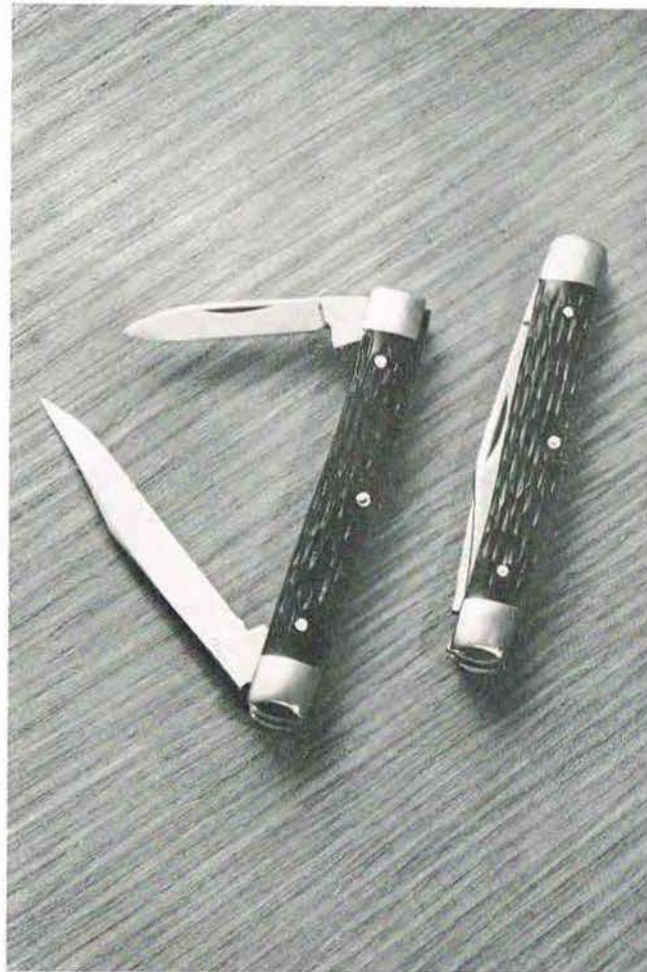
No. 43 Small Two Blade Serpentine Pattern — Staggered handle. Made of Queen Steel. Will not rust or stain and because of Queen's secret tempering process, it will stay sharp far longer than other knives. Nickel Silver double bolsters, brass linings. 2-inch clip blade with 1\frac{7}{8} -inch cutting edge and 1\frac{1}{4} -inch pen blade with 1\frac{1}{8} -inch cutting edge. 2\frac{5}{8} inches long when closed.
