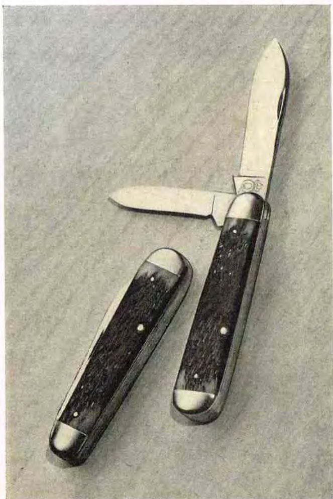
No. 18 Spear Point Special — Two-blade jack knife. Genuine bone stag handle. Double bolster, brass lined, nickel silver finish. One spear point blade is 2\frac{11}{16} inches long and one pen blade 2\frac{3}{16} inches long. 3\frac{11}{16} inches long when closed. Textile workers and mariners prefer this number.
